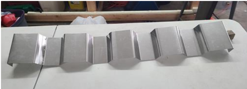
Figure 12. Heat absorbing fin prior to install (unpainted)
